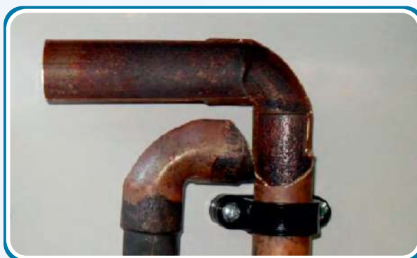
Brazing without Inert Gas Shield
